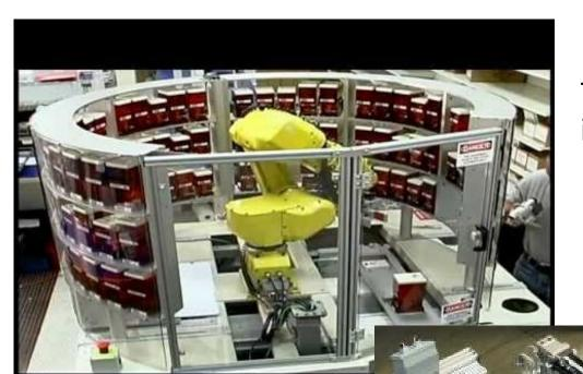
High flexibility robotic filling into vials deposited in totes
