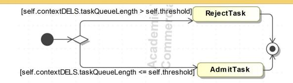
Need a specification of the function required to execute the *AdmitTask(*) behavior
